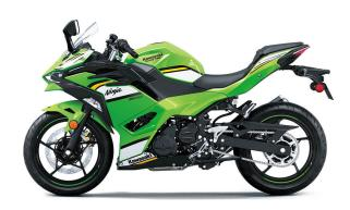
Single 310mm semi-floating disc with 2-piston
